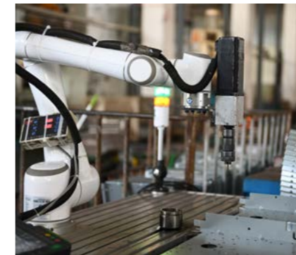
Drilling of metal sheets
